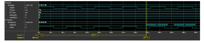
The block accepts input only when the **ready** is 1 (high). In this case, the block captures parameters on the first cycle when the input **valid** port is 1 (high).
