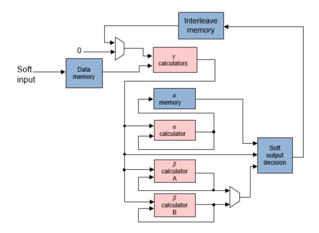
In a normal BCJR architecture, the algorithm cannot compute  $\beta$  until the entire frame is in memory. It must perform a full-frame forward trace and then a full-frame backward trace, which means the latency of one half-iteration is two frame lengths. The required memory is *BlockSize\*NumStates\*DataWidth*. In this case, *NumStates* is eight, from LTE standard TS 36.212 [1].
