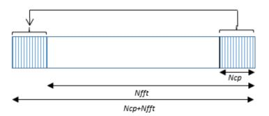
When the OFDM Modulator block operates through Input portselection, it uses the **Maximum FFT length** parameter to avoid multiple IFFTs.
