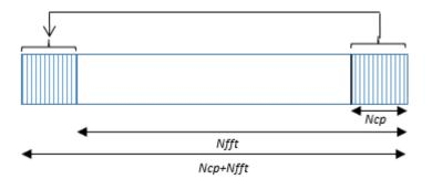
The LTE OFDM Modulator block uses FFT size of 2048 for all NDLRB resources to avoid multiple IFFTs. The block uses CP values corresponding to NDLRB 100.
