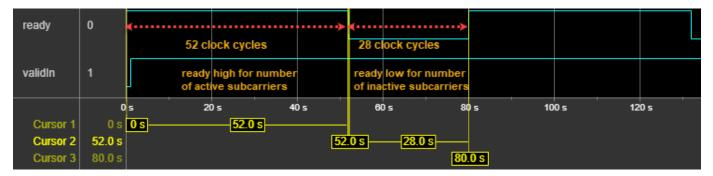
This figure shows the ready signal generation for the default block configuration (**FFT length** = 64, **Cyclic prefix length** = 16, **Number of left guard subcarriers** = 6, **Number of right guard subcarriers** = 5 and **Insert DC Null** = on) with a four-element column vector input.
