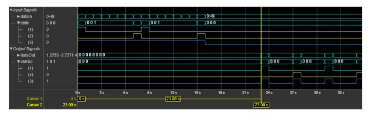
This figure shows a sample output and latency of the block when you set the **Modulation source** parameter to Input port and the **modIdx** input port to 4 (pi/2-BPSK), and 0 (QPSK), and then 1 (8-PSK). The latency of the block varies with the modulation selection. The latency of the block is 27 clock cycles.
