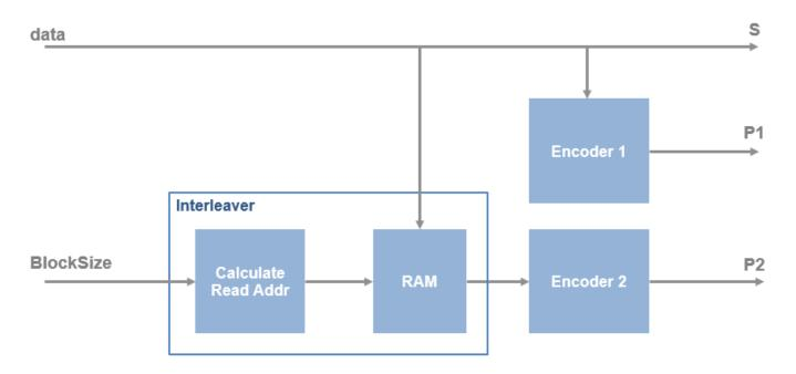
Therefore, the block stores  $f_1$  and  $f_2$  in memory, and uses those two constants and four adders to calculate the interleave indexes.
