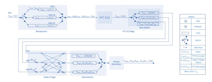
The input sequence x(n) is demultiplexed into three DIT sequences, x(3n), x(3n+1), x(3n+2), each of length 512. Three first-input first-output (FIFO) memories store these sequences. These DIT sequences are serialized and streamed through the **FFT 512** block.
